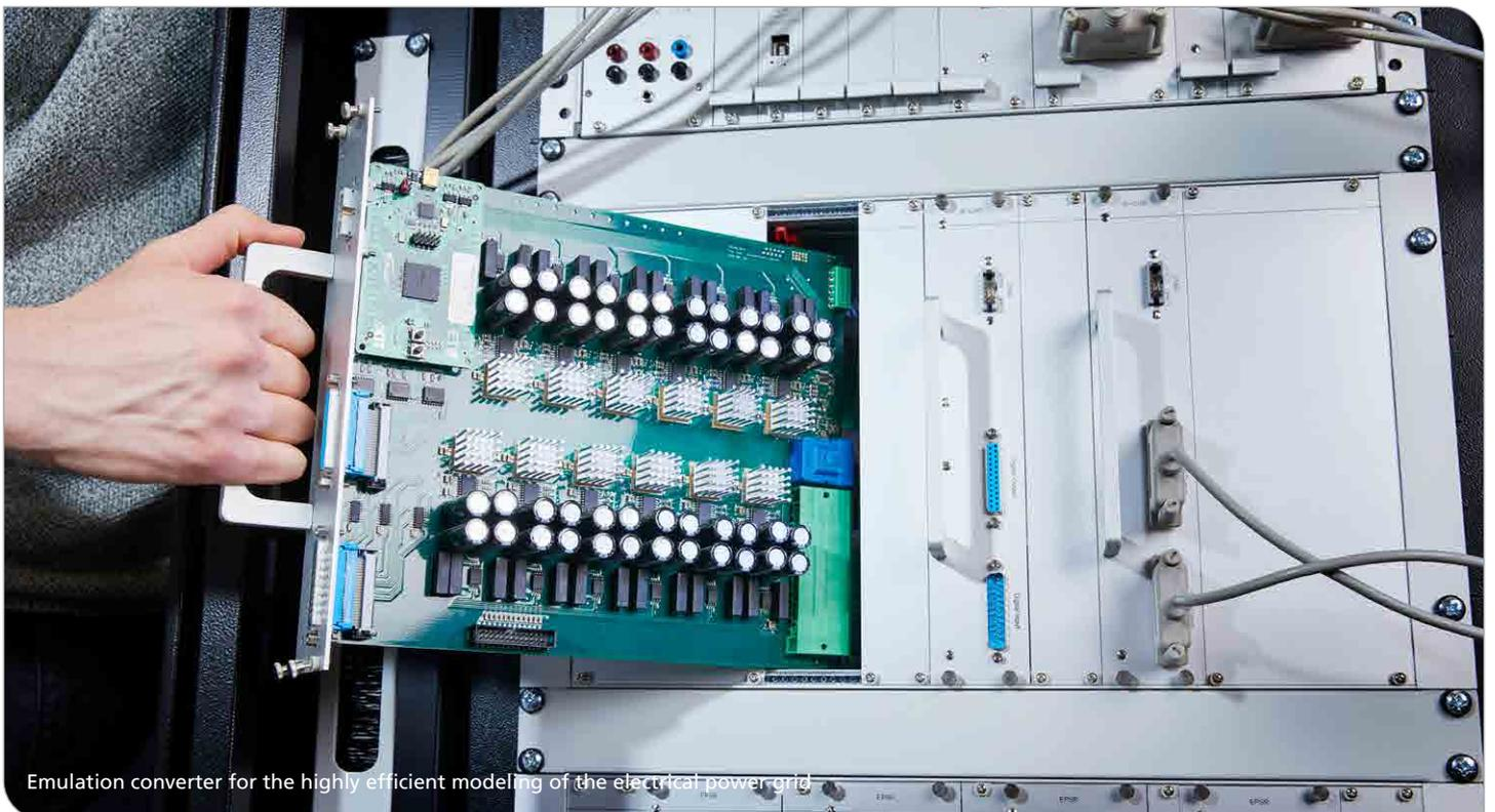
Emulation converter for the highly efficient modeling of the electrical power grid
