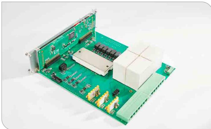
Three-phase module of a two-level converter of 25 kW power
