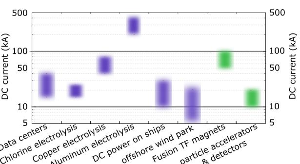
High-Temperature Superconductors (HTS) can improve the energy-efficiency of many industrial high-current DC applications [2]
