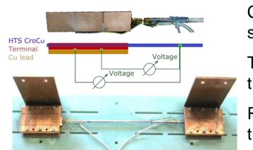
Current is injected to the terminals from the bottom side with leads of same length as the terminals.
