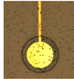
Figure 3: Photograph of a single electrode on top of the porous membrane with insulating layer.
